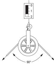
A rope that makes a 90° angle exerts 1-1/2 times the pulling force on the hook and structure.
