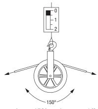
A rope that makes a 150° angle exerts 1/2 of the pulling force on the hook and structure.
