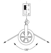
A rope that makes a 120° angle exerts the total pulling force on the hook and structure.
