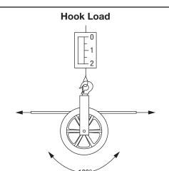
A straight rope exerts no load on the hook and structure.
