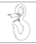
Position latch over tines of spring with ears partially over hook cam. Swing latch to one side of hook, point and depress latch and spring until latch clears point of hook.
