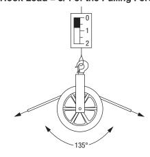
A rope that makes a 135° angle exerts 3/4 of the pulling force on the hook and structure.
