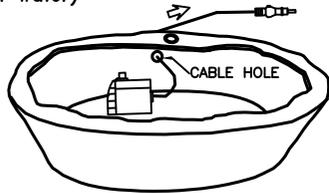
2. FIRSTLY, ATTACH THE WATER HOSE TO THE PUMP, THEN ATTACH THE FROG TO THE WATER HOSE AS DIAGRAM BELOW.
