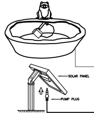
7. INSERT THE SPIKE INTO THE GROUND. POSITION THE SOLAR PANEL TO FACE SOUTH (In Northern Hemisphere) AS MUCH AS POSSIBLE TO MAKE THE MOST OF THE DAYLIGHT HOURS. IT IS IMPORTANT TO ANGLE THE SOLAR PANEL TO FACE SUN WHEN SUN IS AT ITS HIGHEST POINT. ENSURE THE SOLAR PANEL IS NOT SHADED BY TREES, SHRUBS OR BUILDINGS.
