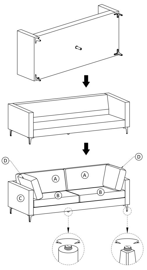
Note: Levelers on bottom of legs can be adjusted if floor is uneven.
