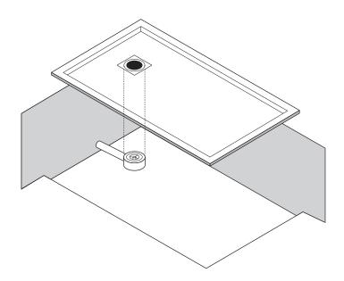
· To ensure a leveled finish using the mortar compound, make sure that the hole around the drain is not higher than 2 cm and is not below base level.
