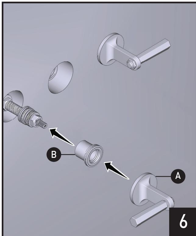
Install the handle valve adapter, Valve Flange (x2) (B), and Handle (x2) (A), onto the shortened valve threads (x2).
