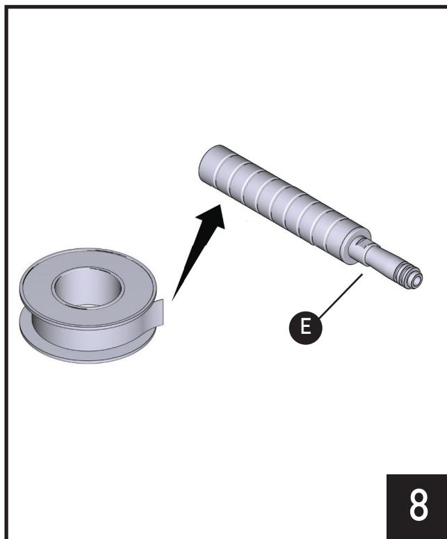
Wrap Thread Seal Tape 3 turns around end of Spout Stem Adapter (E).
