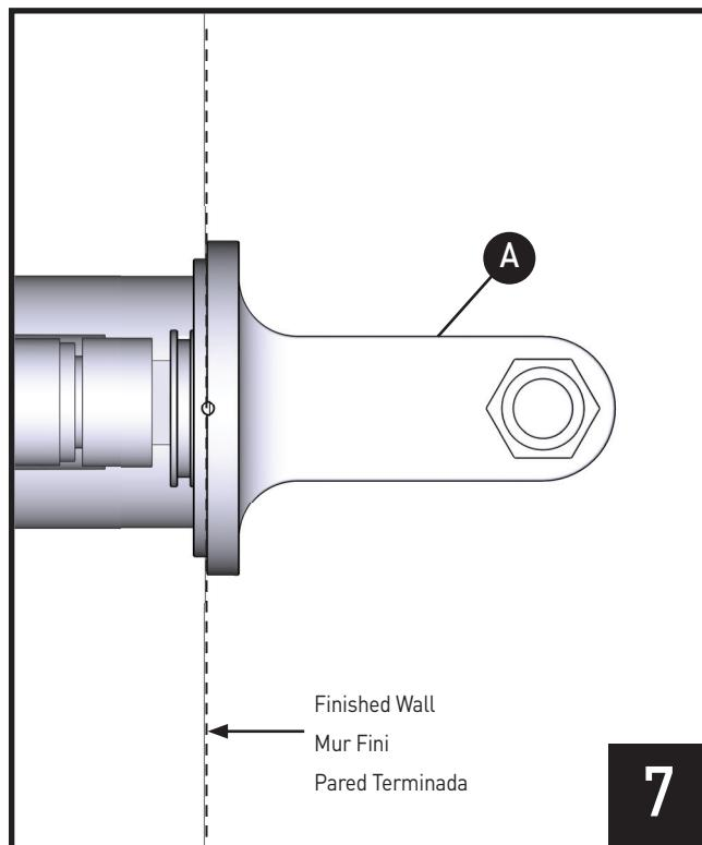
Handles (A) should now be flush with finished wall.
