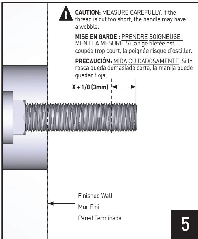
Once measurement is defined, carefully use a hacksaw to trim off the extra threads.
