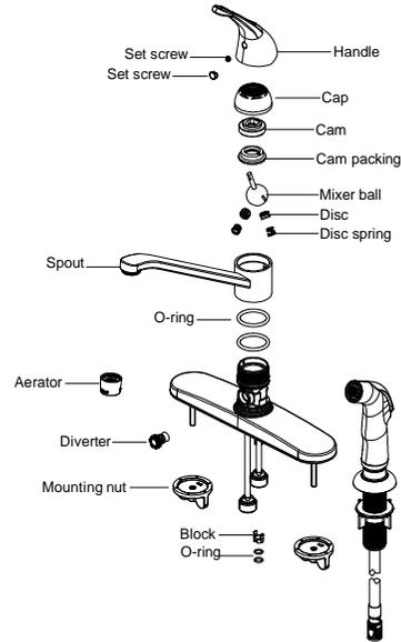
Many of these parts come preassembled. This exploded diagram is to assist in trouble shooting.
