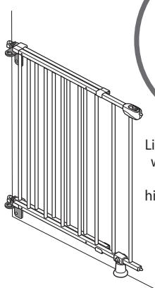
Line the Bolt Assembly up with the hinge as shown.
