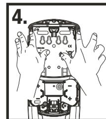
Press firmly on back plate for 10 seconds. For maximum adhesion, do not load refill for 24 hours.
