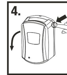
4. Open the dispenser by pushing in one of the dual side latches until it releases.
