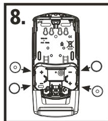
Install 4 fresh D-cell alkaline batteries according to diagram shown on dispenser.
