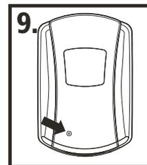
Close dispenser. Battery indicator light will initially alternate blinking red and green. After a few moments, indicator light will consistently blink green when the refill is properly loaded.
