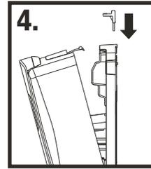
4. To open a locked dispenser, insert key into the key hole on the top of dispenser.
