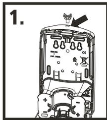
1. Open the locked dispenser by inserting the key into the key hole on the top of dispenser.
