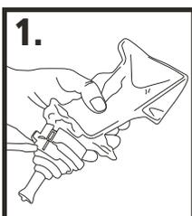
Insert a flat blade screwdriver into the slots on the refill collar and twist to separate the collar from the refill. Unscrew the pump from the bottle and discard.
