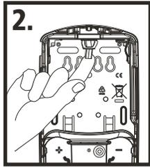
2. To lock the dispenser, remove key from the key mount on the inside of the dispenser.
