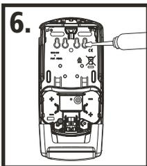
Using back plate as a template, press a pencil through the installation tape to mark holes. Mark and drill holes. Install with #10 x 1" anchors and type A #10 x 1" screws.
