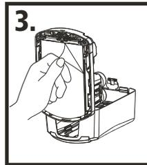
Clean installation surface with an alcohol pad. Allow surface to dry for 60 seconds. Peel paper off installation tape.
