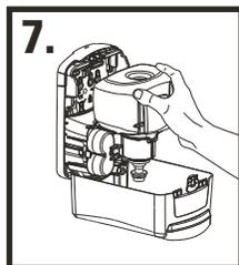
Remove cap from refill pump. You will notice a small knob (E-key) protruding from the white pump collar – **DO NOT REMOVE THIS E-KEY** as its removal will prevent the refill from dispensing. Push refill with E-key facing the back plate, into pump house.
