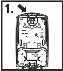
1. The key to lock the dispenser is located in the key mount on the inside of the dispenser.
