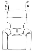
**Step4** Attach the leadwires found at the bottom of motion back to the leadwires at the rear of seat. Yellow to Yellow & Grey to Grey. Make sure to close the clip locks to assure the connections will not come loose during use.
