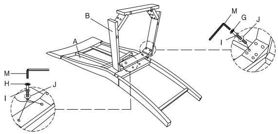
Take the Allen Key, and turn the bolts until the legs are secure. DO NOT TIGHTEN COMPLETELY.
