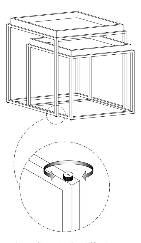
**Note:** Levelers on bottom of legs can be adjusted if floor is uneven.
