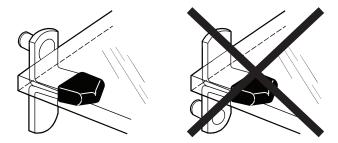
2. The electrical cord was installed at our factory and should remain along the inside of the cabinet.
