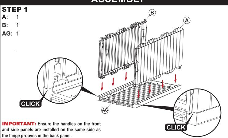
Firmly and evenly press Front Panel (A) and Back Panel (B) into one Side Panel (AG).
