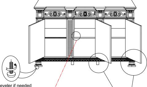
Step 4: Adjust Leveler if needed to level case on uneven floor.
