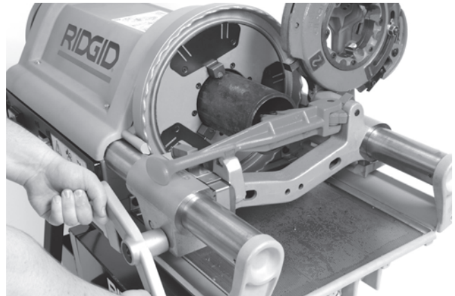
Figure 22 – Reaming Pipe with Reamer
