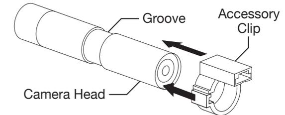
2. Position accessory in the groove near the middle of the camera body.
