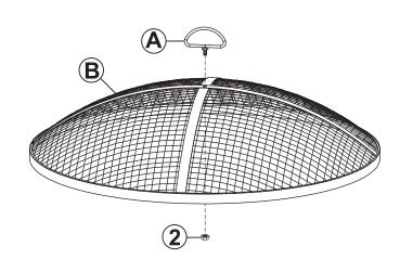
Align Handle (A) with Spark Screen (B) and firmly securing using one Nut (2).
