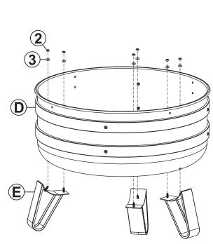
Align one Leg (E) with the bottom of Fire Bowl (D) and firmly secure using two Washers (3) and two Nuts (2). Repeat to secure the remaining two legs.
