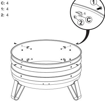
Align one Bracket (C) with the inside of the fire-bowl and secure using one M6x15mm Bolt (1) and one Nut (2). Repeat to secure the remaining three brackets.
