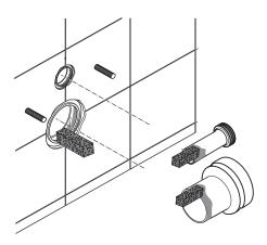
$\cdot$  Use slotted end of thread bolt to adjust in or out. Do not damage the thread.
