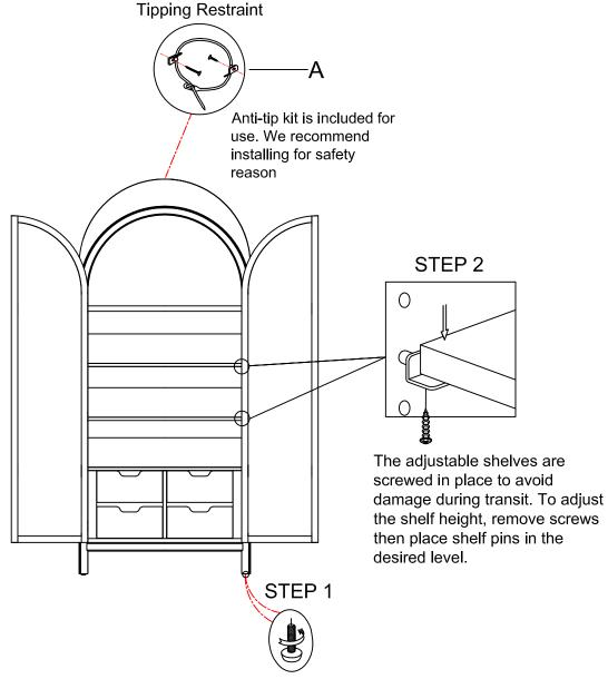
Adjust Leveler if needed to level wardrobe on uneven floor.
