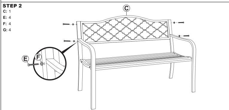
Align Backrest (C) with the top of the side panels and secure using four M6x55mm Bolts (E) and four Washers (F).
