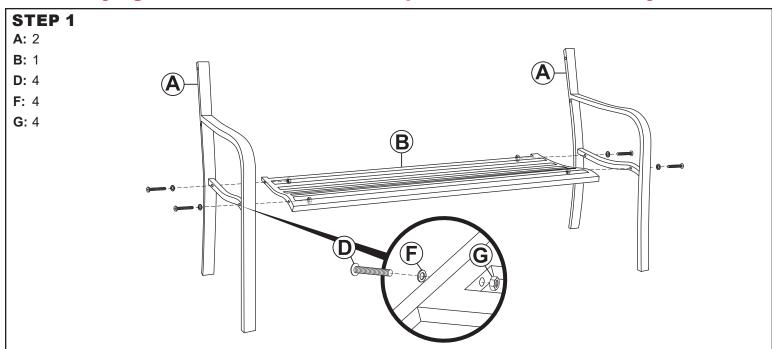
Align one Side Panel (A) with Seat (B) and secure by hand-tightening two M6x50mm Bolts (D), two Washers (F) and two nuts (D). Do not fully tighten hardware until the backrest is secured in the next step.
