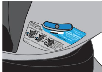
16. For **FORWARD-FACING** installation, Car Seat should be fully upright.
