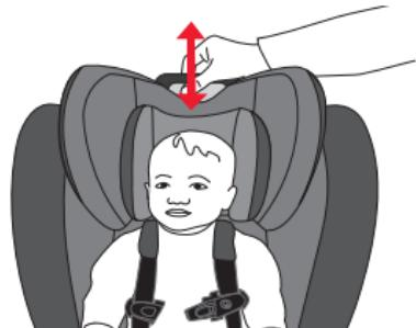
**NOTE:** The Headrest Flap is designed with three fold lines to allow for partial or full storage. If using the lower Headrest/Harness positions, make sure to tuck the excess Headrest Flap up behind itself.
