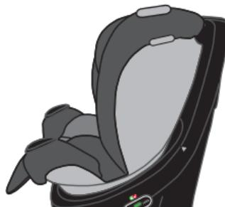
2. Before placing Car Seat in vehicle, remove Seat Shell from Base (see pg. 54).
