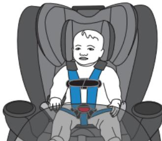
**NOTE:** Child's Head MUST be 2.5 cm (1 in) or more below the top of the Headrest or shell, whichever is higher.
