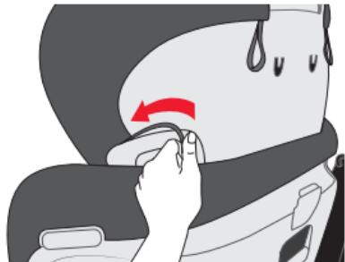
4. Pull the harness strap out of the opening in the headrest pad, and remove headrest pad from seat.
