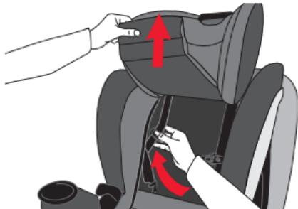
4. Disconnect hook-and-loop connectors attaching seat pad to back pad.
