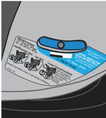
For **REAR-FACING** installation, Recline Ball should be in correct zone for child size:
