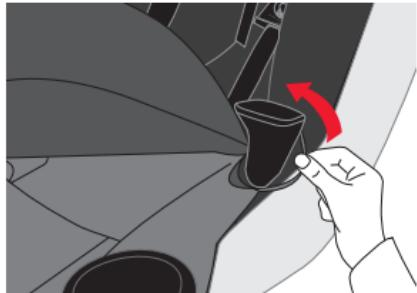
10. Push Buckle and harness adjustment strap throughs slot in seat. Remove seat pad from seat.
