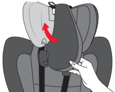
9. Replace the elastic straps at the back of the headrest and around the shoulder belt guides.
