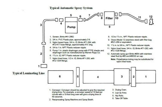
\*To measure fluid flow: Pressurize fluid source only; pull trigger; flow material into measuring device for 60 seconds; increase or decrease fluid source pressure to obtain desired fluid flow.
