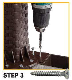
Firmly fasten (4) M6.3x32 sheet metal screws to the sides of each leg.
