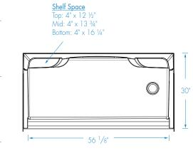
FEATURES Dimensional Tolerance ± 3/8". Dimensions needed for site preparation should be measured from the unit. Manufacturer assumes no responsibility for preparatory work.
