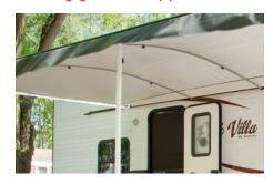
Awning ground support can be added to any existing awning for extra stability when the awning is fully extended. Stabilize your awning and prevent the roller from sagging with Solera awning ground support
