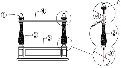
Step 2: Put bottom panel (4) onto the posts (2), then attach feet (1) to posts (2) through bottom panel (4).
