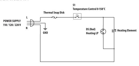
This circuit diagram has been provided to assist qualified electricians; only WINCO service agents or qualified electricians should carry out repairs if required.
