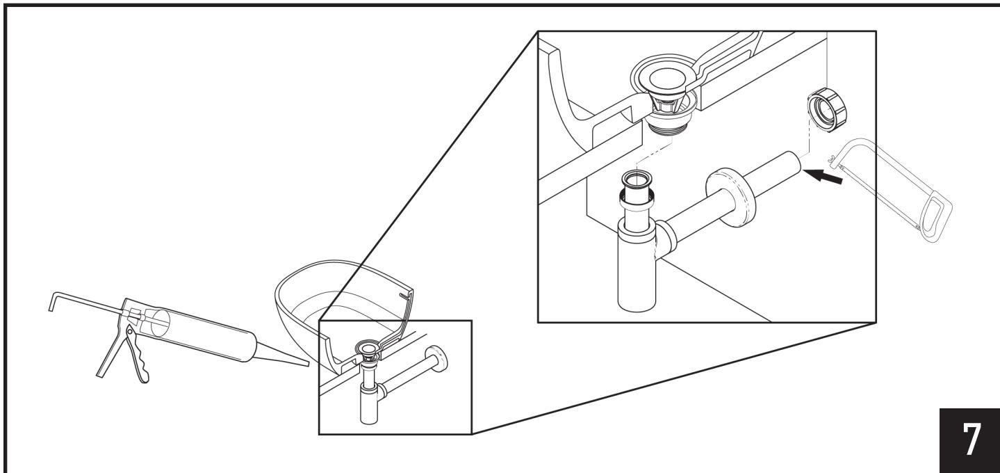
Install appropriate waste drain. Apply Silicone (not provided) to drain waste to secure.
