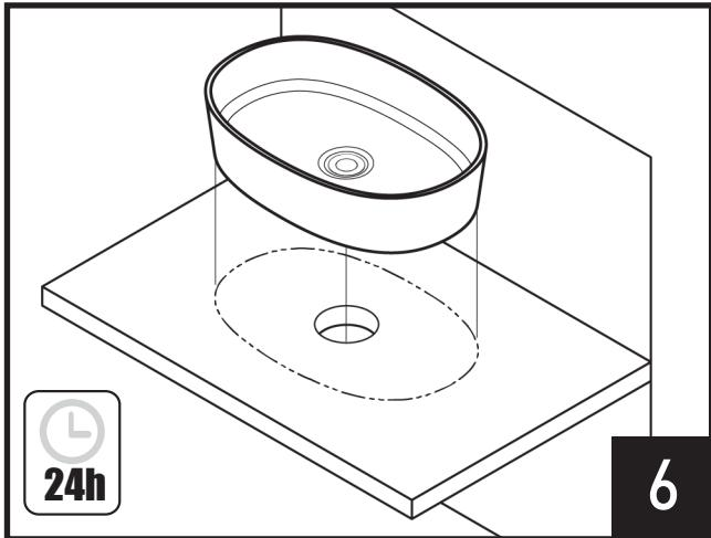
Apply sink to surface. Wait 24 hours for sink to fully secure to surface.
