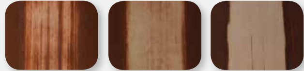
Panel A Traditional Degreaser Dilution Rate 1:40 Scrub Test Cycles: 75
