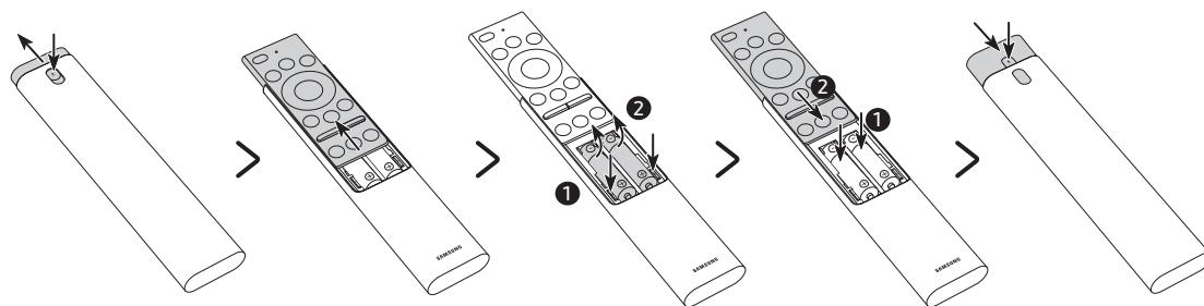
1. Press the
