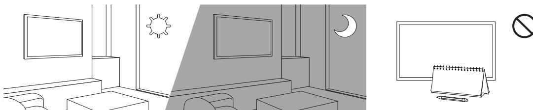
Eco Sensor adjusts the brightness of the TV automatically. This feature measures the light in your room and optimizes the brightness of the TV automatically to reduce power consumption. If you want to turn this off, go to (Home) > Settings > General > Eco Solution > Ambient Light Detection.
