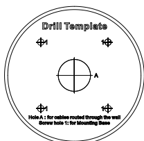
Figure 2-9 Drill Template of the Junction Box
