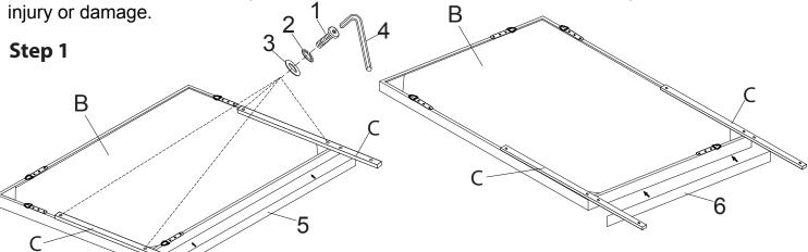
For vertical use, stick felt strip (5) on the vertically bottom of Mirror (B). For horizontal use, stick felt strip (6) on the horizontally bottom of Mirror (B).
