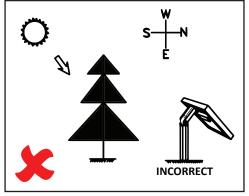
Insert the spike into the ground. Position the solar panel to face South (in northern hemisphere) to make the most of daylight hours. It is important to angle the solar panel towards the sun when sun is at its highest point. Ensure the solar panel is not shaded by trees, shrubs or buildings.
