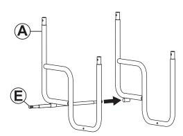
Slide Axle (E) through the holes on the bottom of Base Panels (A).
