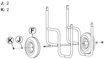
Firmly secure two Wheels (F) to the axle using two M12 Washers (J) and two M12 Lock Nuts (K).
