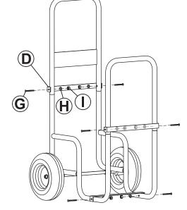
Loosely secure one Brace (D) to the bottom of the log cart by hand-tightening two M8x40mm Bolts (G), two M8 Washers (H) and two M8 Lock Nuts (I).
