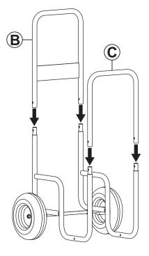
Slide Handle (B) onto the back of the base panels. Slide Log Retainer (C) onto the front of the base panels.
