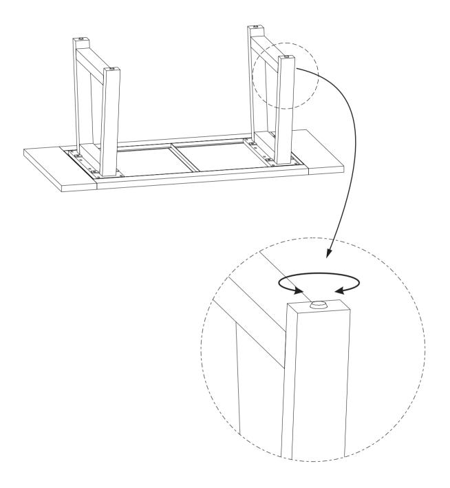
**Note:** Levelers on bottom of legs can be adjusted if floor is uneven.
