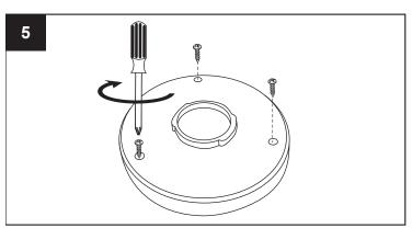
Carefully replace the bottom of the panel and align the screw holes. Secure the panel with the screws removed in step 3. Do not over-tighten the screws.
