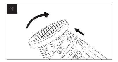
Twist the solar panel counterclockwise and gently lift the panel off the umbrella. Take care not to pull on the wires.
