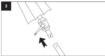
Attach Umbrella (A) to Pole (B) by pushing the button spring clip on the pole and aligning it with the hole on the umbrella. You will hear a 'snap' when the pieces are connected.
