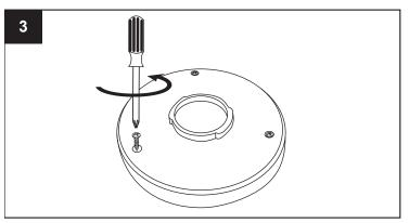
Place the solar panel face-down on a soft, clean surface. Remove (3) screws from the bottom of the panel.
