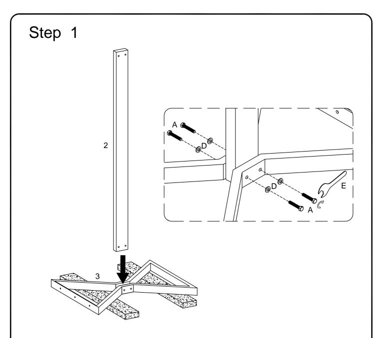
Insert part (2) to part (3) ,then using bolt (A) attach flat washer (D) into part (3) to part (2) with wrench (E) as per diagram.
