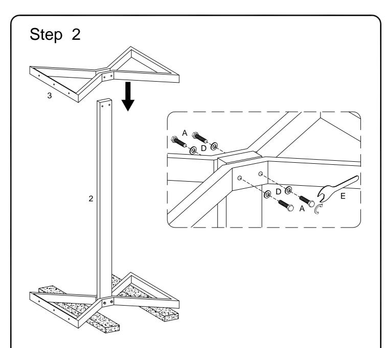
Place part (3) to part (2) ,then using bolt (A) attach flat washer (D) into part (3) to part (2) with wrench (E) as per diagram.
