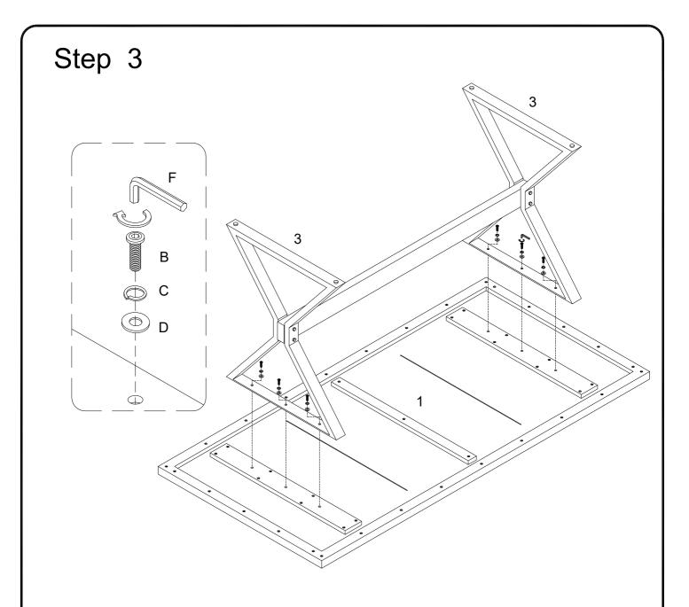
Using bolt (B) attach Lock washer (C) and Flat washer (D) into part (3) to part (1) with Hex key (F) as per diagram.
