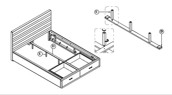
STEP 4: SECURE THE SLAT ROLL (F) TO THE BED ASSEMBLY WITH SIX M4X30 WOOD SCREWS .
