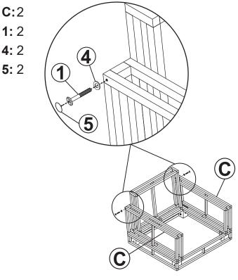
Do not fully tighten hardware until after Step 3 is complete.
