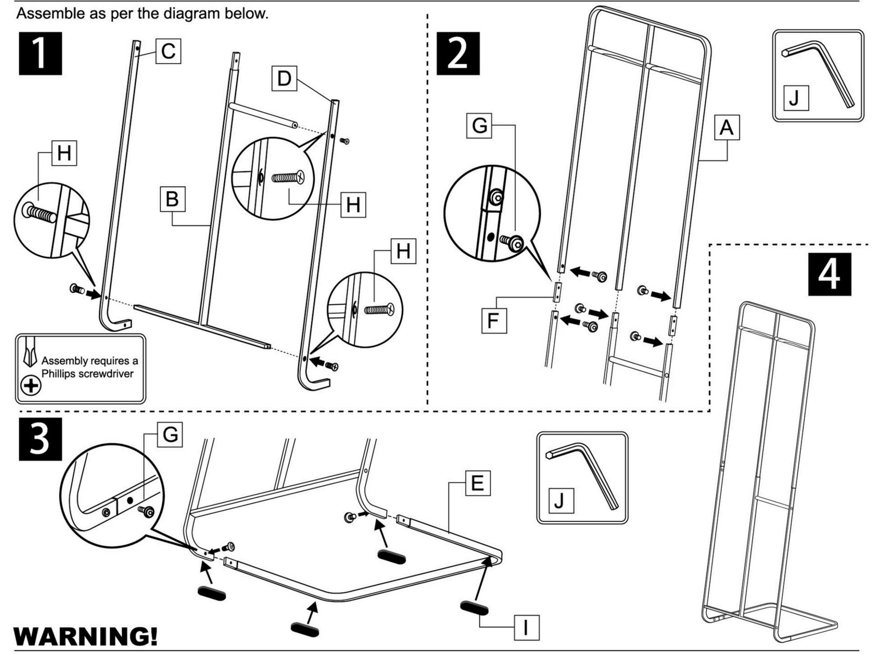
Max loading weight 8lbs (4kg)×2%Top bar 6lbs(3kg)%Bottom bar
