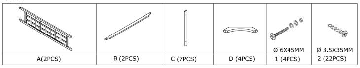
**Step 1:** Attach the two headers (Part B) to the top of the two side lattices (Part A). Use the four included bolt sets (Hardware 1) to attach the two headers to the side lattices as shown in the diagram to the right.
