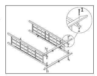
**Step 2:** Attach the seven slats (Part C) to the top of the headers (Part B). Use 14 of the included screws (Hardware 2) to fasten the slats to the top of the headers.
