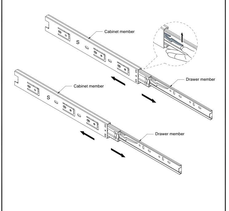
Attach Drawer Glides (S) to the Left Cabinet Panel (8) and Right Cabinet Panel (9) using 12mm Screws (N). Insert Wooden Dowels (A) into side dowel holes.
