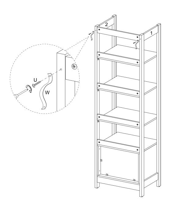
Insert the Wall Anchor (V) into the wall. Next, secure the Plastic Strip (W) to the wall using the 25mm Screw (T).
