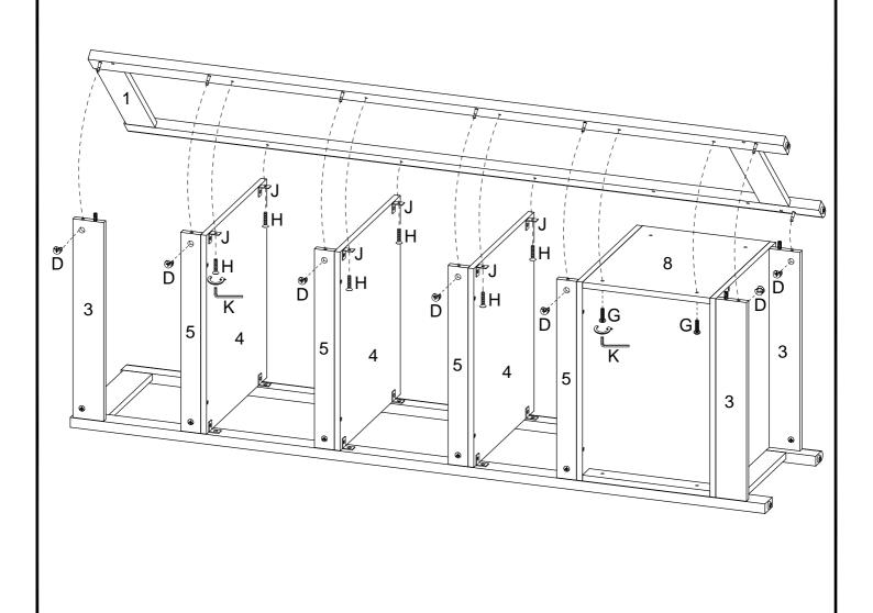
Attach the front of the Left Drawer Panel (8) and the Right Drawer Panel (9) using 30mm Bolts (G).
