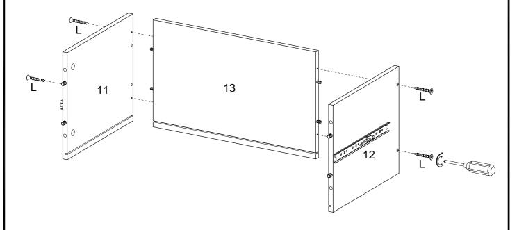
Slide in the Bottom Drawer Panel (10) using the guides. Attach Front Drawer Panel to the Left Drawer Panel (11) and Right Drawer Panel (12) using Cam Locks (E).
