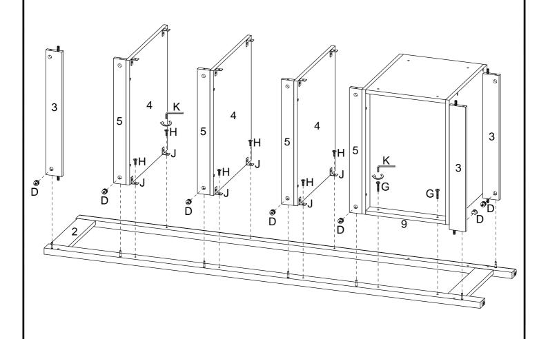
Repeat these steps for the other side. Attach Front Shelf Trim x4 (5) & Support Panels x3 (3) with Cam Locks (D). Secure with screwdriver. Next, attach L Shape Brackets (J) on Upper Shelf Panels (4) to the Left Side Panel (1) using 15mm Bolts (H). Lastly, connect the Left Cabinet Panel (8) to the Left Side Panel (1) using 30mm Bolts (G).
