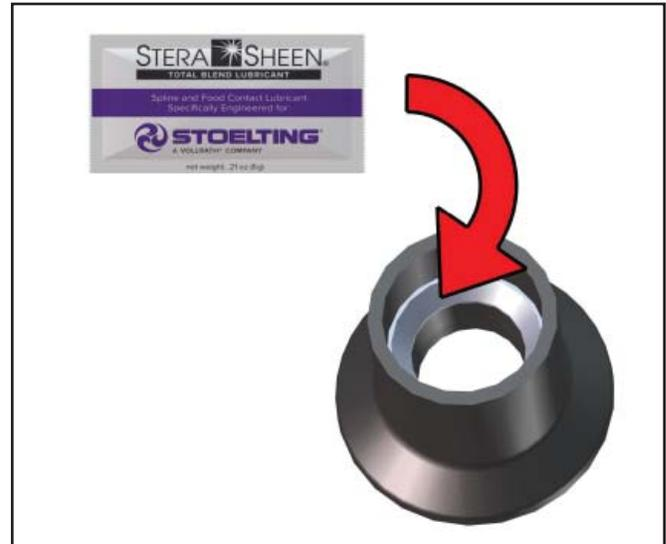
Figure 3-5 Lubricate Rear Seal
