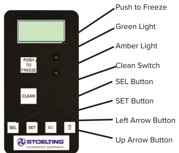
Figure 3-2 IntelliTec™ Control
