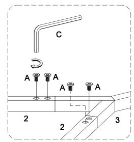
Insert part (3) into legs (2), then use wrench (C) to secure them with bolt (A).
