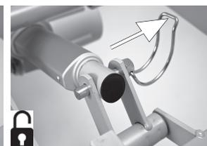
Fold out the clamp and pull out the pipe pin.
