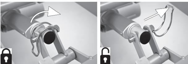
Push the cotter pin through motor and attachment. Fold the clamp over the pin. The motor is now secured.
