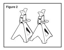
stands simultaneously under both ends of vehicle or under one side of vehicle.
