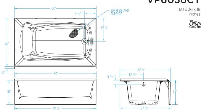
FEATURES Dimensional Tolerance ± 3/8". Dimensions needed for site preparation should be measured from the unit. Manufacturer assumes no responsibility for preparatory work.
