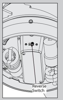
**Changing the direction of air flow** - carefully remove the globe and move the reverse switch to the opposite position. Reinstall the globe.
