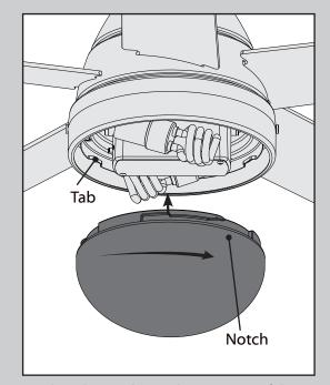
Align the notches in the outer rim of the globe with the tabs on the light kit assembly Carefully lift the globe up inside the light fixture as far as it will go. Rotate the globe in a clockwise direction until it is held tightly in place by the three tabs.
