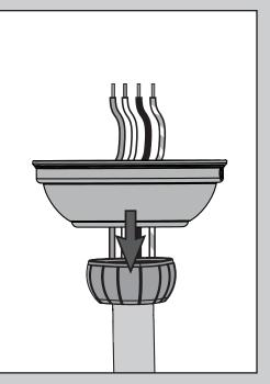
Put the wires and downrod through the canopy. Let the canopy sit loosely on top of the fan.
