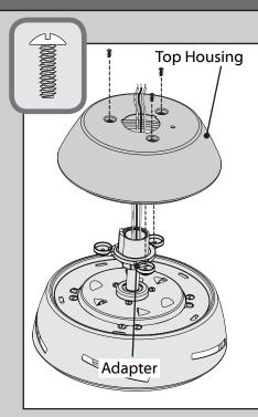
Thread the wires through the top housing. Place the top housing onto the motor housing so that the holes in the top housing lineup with the holes in the motor housing and the adapter. Install the three top housing screws.
