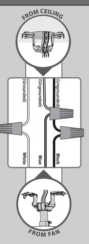
Turn the splices upward and push them carefully back through the hanger bracket into the outlet box. Spread the wires apart, with the grounded wires on one side of the outlet box and the ungrounded wires on the other side of the outlet box.
