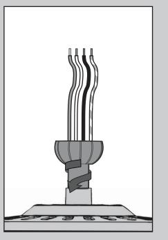
Hand tighten the downrod (at least 4-5 full turns) until it stops.
