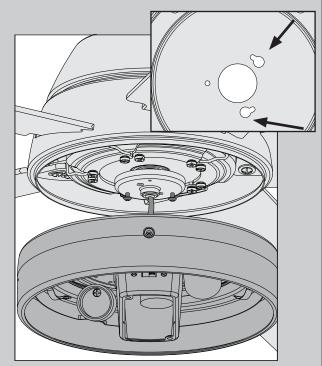
Align the keyhole slots in the top of the light kit assembly with the partially installed assembly screws. Wrap the keyhole slots around the screws and twist counterclockwise.
