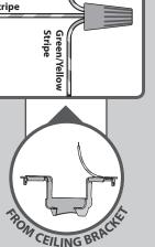
Note: To connect the wires, hold the bare metal leads together and place a wire connector over them, then twist clockwise until tight.
