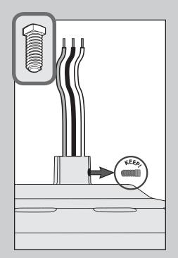
Remove the pre-installed setscrew so that the downrod can be inserted.
