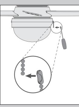
Remove and discard the plastic connectors from the ends of the short pull chain. Connect the appropriate pull chain pendant to each of the short chains. The fan pull chain controls the speed: from high to off. The light pull chain controls the light fixture: on and off.
