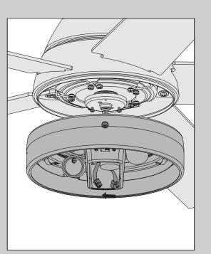
Feed the 9-pin plug connector coming from the bottom of the motor housing through the center hole in the light kit assembly. Connect it to the plug connector found in the switch housing area of the light kit assembly. Make sure to line up the colored markings on the connectors.
