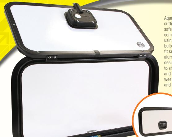
Aqua Shed Baggage Doors are the cutting-edge in water management, safeguarding RV exterior compartments from water infiltration using automotive-grade, low-profile bulb seals with radius corners that fit snugly into the heavy-duty radius aluminum frame. The watertight design uses an outer frame drip rail to shed water away from the hinge and an internal extruded channel and weep holes to drain excess water off and out. Aqua Shed Baggage Doors feature pre-punched interior
