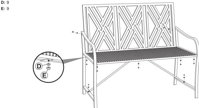
Secure all components using nine Washers (D), and nine Cap Nuts (E), as shown.
