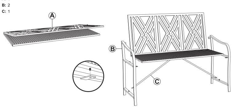
Align Rod (C) with the weld screws on the bottom of two Side Panels (B), as shown. Then, align the weld screws on Seat (A) with the side panels.
